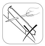
If the cutterblade is not balanced the heavy end will rotate downwards. Sharpen the heavy end until the cutterblade is correctly balanced.
